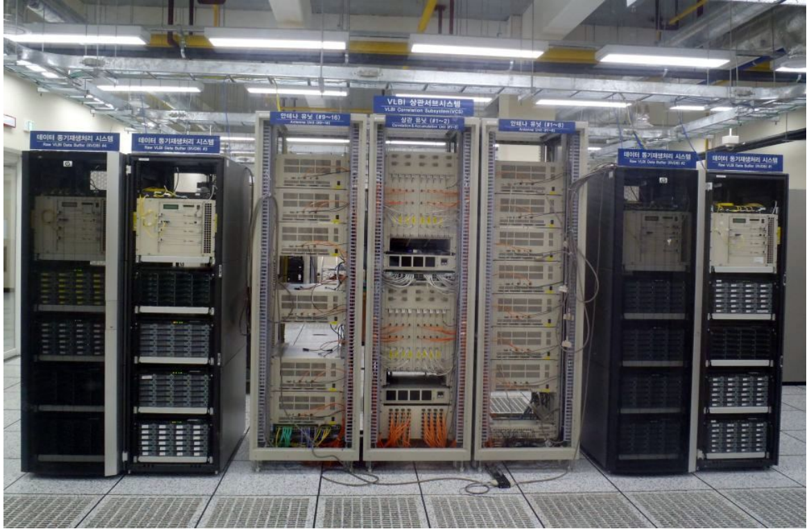
Figure 16: Daejeon Correlator installed at Korea-Japan Correlation Center
