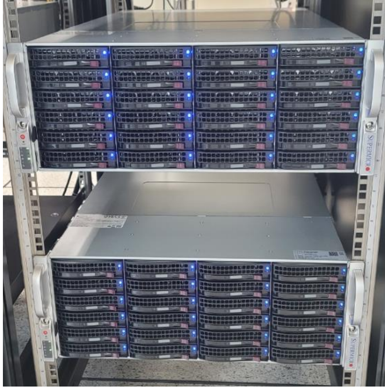
Figure 16: Front view of the two Flexbuff units at KPC. 24 disks are mounted for one Flexbuff.
