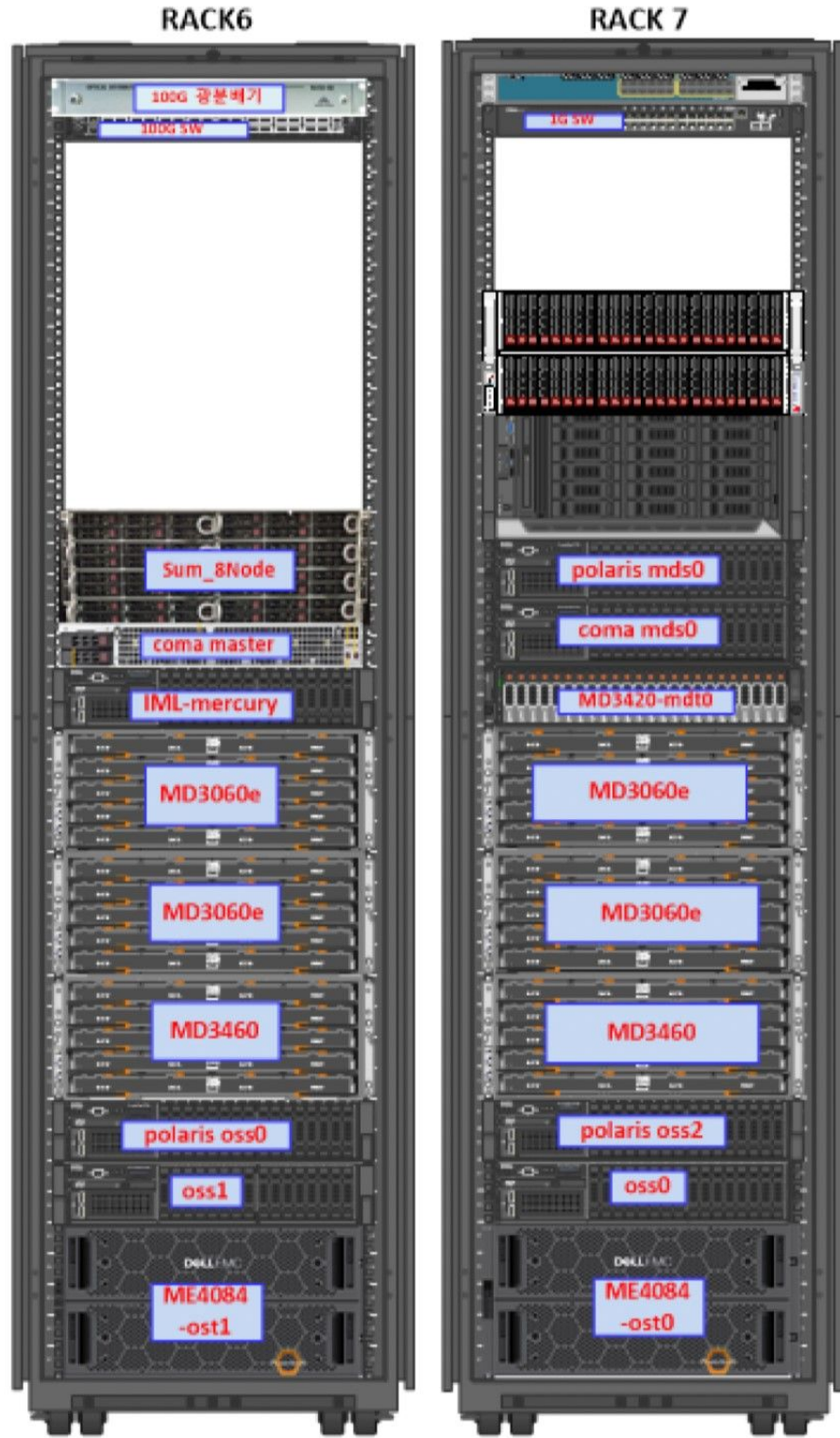
Figure 18: A computing cluster and Lustre file system dedicated for the software correlation of the KVN.
